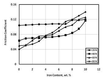
Fig. 12 Friction coefficient of epoxy composites sliding against water/oil emulsion lubricated rubber.
