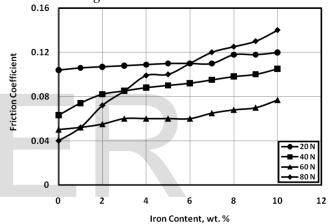
Fig. 10 Friction coefficient of epoxy composites sliding against oil lubricated rubber.
