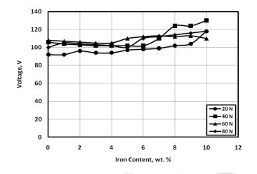
Fig. 7 Voltage generated from epoxy composites sliding against detergent wetted rubber.
