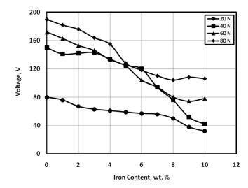
Fig. 9 Voltage generated from epoxy composites sliding against oil lubricated rubber.
