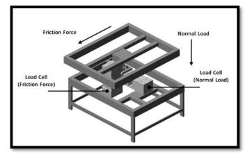
Fig. 1 Details of the test rig.
