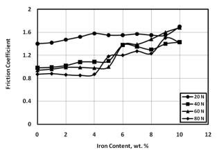
Fig. 4 Friction coefficient of dry sliding of epoxy composites against rubber.
