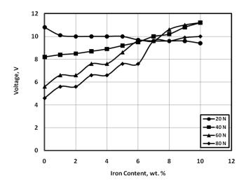
Fig. 11 Voltage generated from epoxy composites sliding against water/oil emulsion lubricated rubber.
