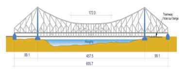
Figure 1. Schematic Elevation of Howrah Bridge
