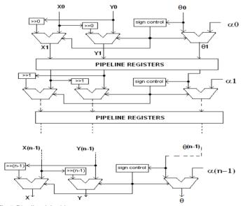
Fig.5 Pipelined Architecture
