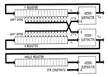
Fig.2 Basic Arithmetic Unit for CORDIC Algorithm
