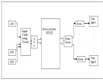
Fig 1.2 Block diagram of developed lighting control system
