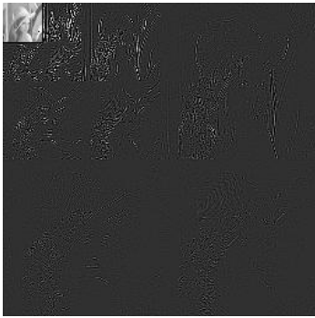
Fig.3. Three layer decomposition of the 'Lena' image.
