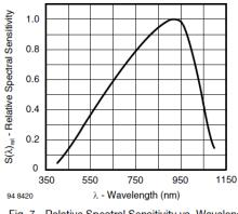
Fig. 7 - Relative Spectral Sensitivity vs. Wavelength
