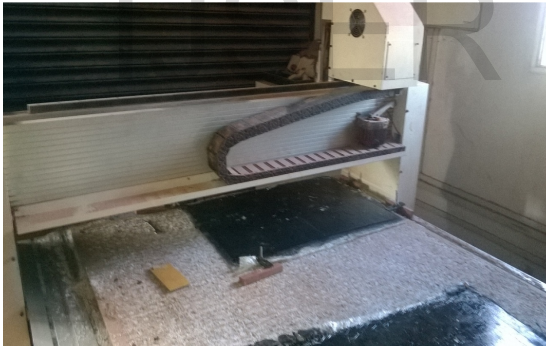
Fig 5.6 cutting of carbon fibre using CNC
