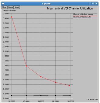
Fig. 10 Comparison of Mean arrival VS Channel utilization using normal spectrum utilization and Fuzzy Logic
