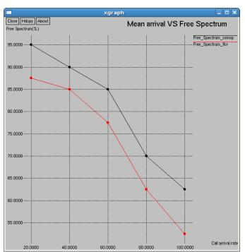
Fig. 5 Comparison of Mean Arrival VS Free Spectrum using normal spectrum utilization and Fuzzy Logic
