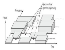
Fig. 1 The Spectrum Hole Concept
