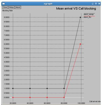
Fig. 4 Comparison of Mean Arrival VS Call blocking using normal spectrum utilization method and Fuzzy Logic System
