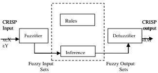
Fig. 2 The Structure of a Fuzzy Logic System
