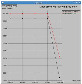
Fig. 9 Comparison of Mean Arrival VS System Efficiency using the normal spectrum utilization and Fuzzy Logic System
