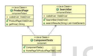
Fig. 3. The UML Class diagram showing ProductPage an d searchBar with ComponentTests.
