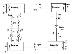
Figure 1: Schematic Diagram of Simple Vapour Absorption Refrigeration System
