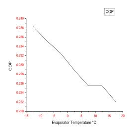
Figure 5: Variations of COP with Evaporator Temperature Effect of Effectiveness of Heat exchanger on Coefficient of Performance:-
