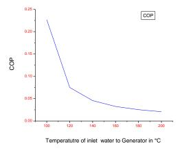
*Figure 3: Variations of COP with inlet water temperature to Generator* (*T*<sup>11</sup>)
