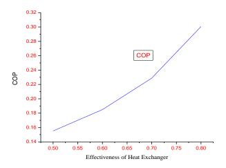
Figure 6: Variations of COP with Effectiveness of Heat Exchanger
