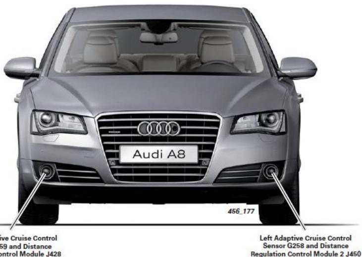
Fig.3 Front View of vehicle with ACC Sensors
