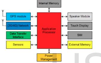
Fig. 2. General architecture of a modern smartphone. and video camera [34]. The ARM Cortex-A chips series introduced processors d signed for smartphone applications. The Cortex-A15 MPCore processor is the latest of the Cortex-A series and it is based on ARMv7-A Cortex architecture with processor speed up to 2.5 GHz [35]. Exynos 5 Dual core is the Samsung Galaxy SIII AP, based on the ARM Cortex-A15 processor with clock speed up to 1.7 GHz [36].
