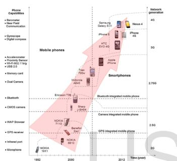
Fig. 1. The evolution of mobile phone vs the number of integrated sensors and the mobile network standard since 1992 to 2012.
