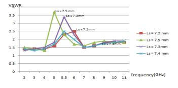
Fig. 4: variation of the simulated VSWR with different slot length (Ls) in the ground plane.
