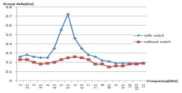
Fig. 7: simulated group delay of antenna with and without notched.
