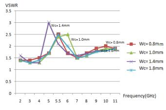
Fig. 6: variation of the simulated VSWR with different location of the slot (
