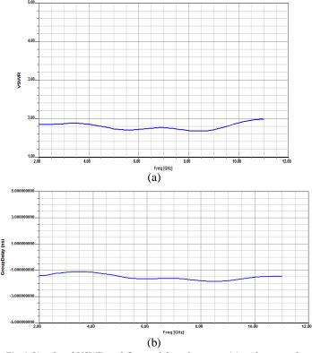
Fig. 2 Simulated VSWR and Group delay of antenna (a) without notch with optimal dimensions.
