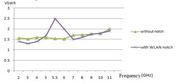
Fig. 3: Simulated VSWR of antenna with WLAN notch and without notch
