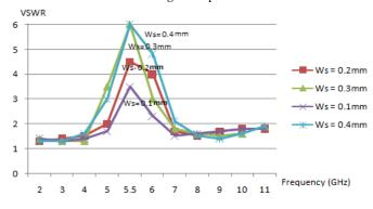
Fig. 5: variation of the simulated VSWR with different slot widths (Ws) in the ground plane.
