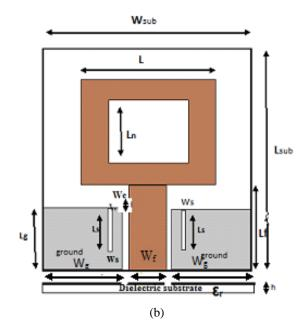
Fig. 1: Geometry of the proposed CPW-fed UWB antennas (a) without notch, (b) with single notch
