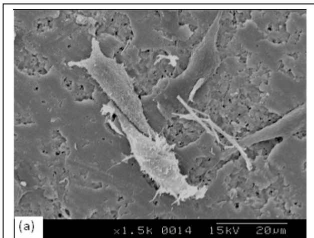
Fig. 6a. SEM micrograph of cellular adhesion URH blocks sintered at 1200°C/2hrs
