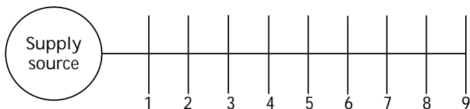
Fig. 2. Testing distribution system with nine buses
